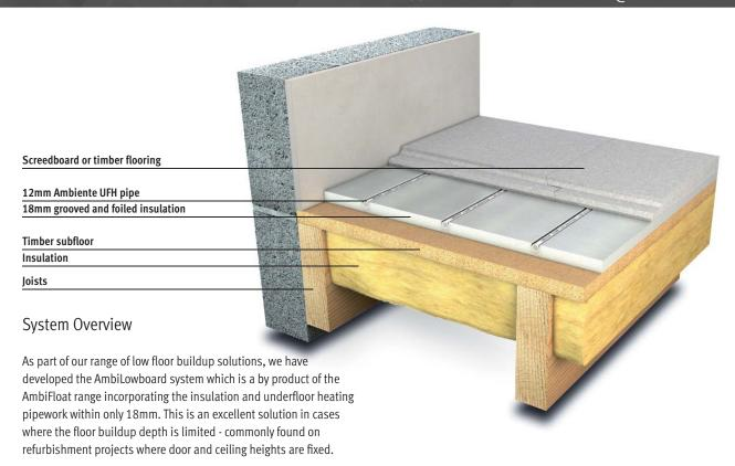
The AmbiLowboard system can be used in existing and new build applications. It requires a flat and level solid sub floor for the insulation to fully support the floor finish on top. The insulation is pre-grooved to take the 12mm underfloor heating pipework and over laid with foil to assist the distribution of heat. The polystyrene insulation panels are manufactured as per the design drawings.
