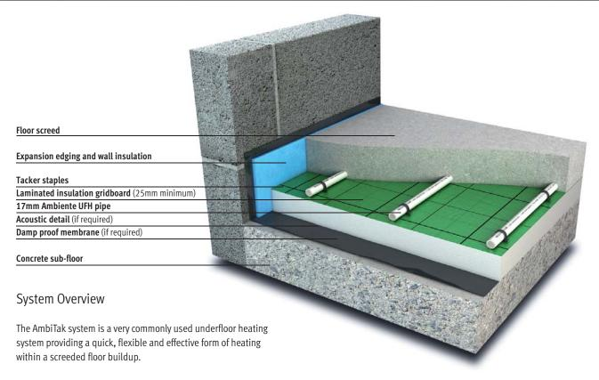
Primarily this system is used in conjunction with the laminated and gridded EPS insulation board. This provides a strong base to fix to and the grid lines act as a guide to help install the pipework at the correct spacings. Edge and floor insulation is installed over the subfloor on to which the underfloor heating pipe is laid and fixed using barbed tacker staples. Where insulation is not supplied, checks should be made to ensure that the insulation is compatible with this system.
