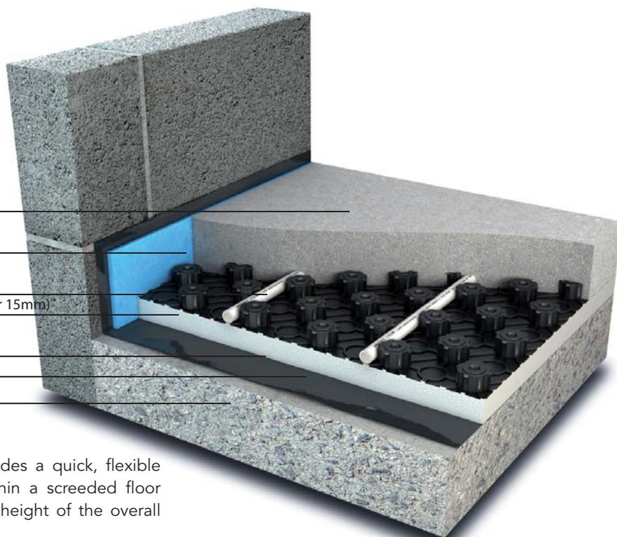
The AmbiCastellated system provides a quick, flexible and effective form of heating within a screeded floor buildup as well as minimising the height of the overall floor construction.
