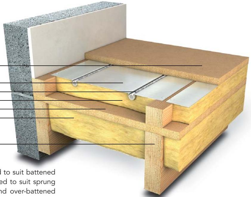
The AmbiPlate 20:1 system is designed to suit battened floor buildups but can be easily adapted to suit sprung sports floors, acoustic batten floors and over-battened floors.
