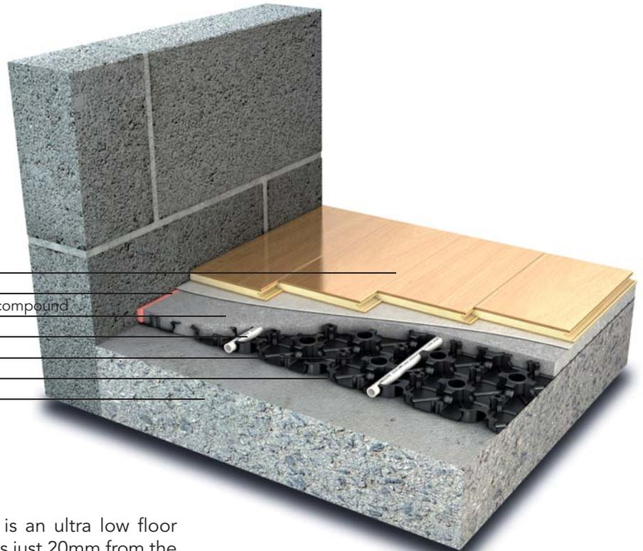
AmbiSolo floor panel system is an ultra low floor build up solution that measures just 20mm from the panel base to the top of the levelling compound. It can be installed on any existing floor construction such as screed, timber joisted or tiled floors. The rear face of the panel has a high strength self adhesive surface that ensures secure positioning on the floor during installation.
